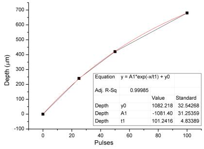
Fig. 3 - Depth of craters (µm) vs. number of laser pulses. The depth of craters follow approximatively an exponential curve.
