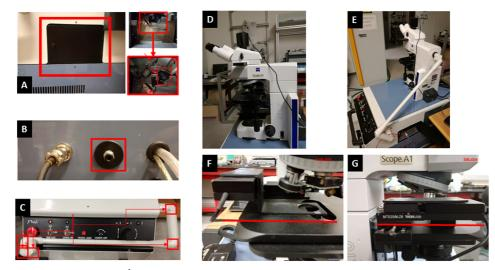
Fig. 1 - The different part of the MODÌ instrument. A) Main analysis chamber with some details; B) backpanel with airflow nozzle; C) external articulated arm with the indication of reflecting mirror positioning; D) the microscope with digital camera; E) the microscope attached to the instrument by mean of the articulated arm; F) scanning system X axis; G) scanning system Y axis.
