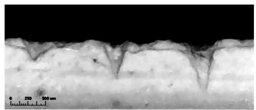
Fig. 2 - Craters made by laser in the analytical chamber. From left to right: after 25, 50 and 100 laser shots.
