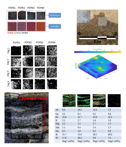
Fig. 4 - Some examples of the capability of the system: elemental maps, false color map (combining different maps), Artificial Inteligence segmentation of the map features and 3D reconstruction of the ablated surfaces.
