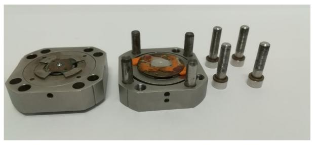
Fig. 2 - Components of an ETH-type diamond anvil cell with the four screws used to load to the diamonds
