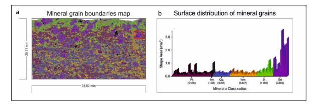
Fig. 3 - Result of the Min-GSD ArcToolbox: a) mineral grain size polygon map. All of the polygons constructed by the GSD toolbox are labelled with the appropriate mineral name classified via the Q-XRMA; b) histogram of grain size frequencies distinct for each mineral.
