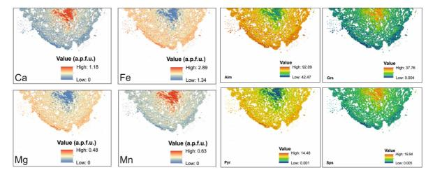
Fig. 2 - Example of Ca, Fe, Mg and Mn calibrated images and component maps derived for a garnet microdomain.
