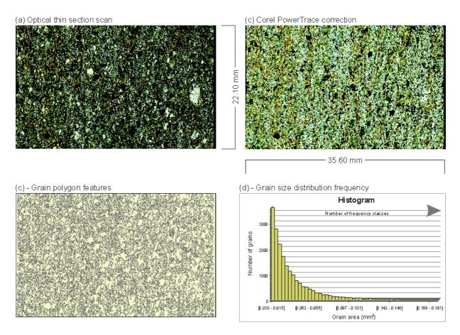
Fig. 1 - Result of the GSD ArcToolbox: a) original optical thin section; b) result of the PowerTrace Function of Corel Draw Software; c) polygon shapefile created via a feature to polygon conversion; d) histogram of the grain polygon as a function of their shape area.
