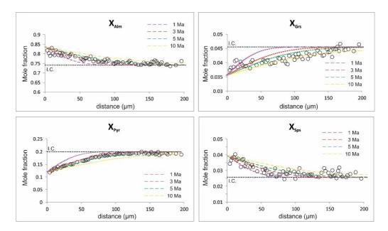
Fig. 6 - Diffusion model of the garnet retrograde zoning.  $X_{Grs}$  shows a longer timescale probable as a consequence of the slower calcium cationic movement.
