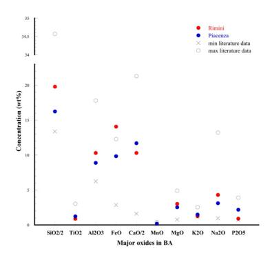
Fig. 1 - Bottom ash compositions, expressed as wt.% oxides for the bottom ashes from Rimini and Piacenza plants compared to various literature sources (min and max are the limits of literature range: Kirby & Rimstidt, 1993; Kida *et al.*, 1996; Barbieri *et al.*, 2000; Ferraris *et al.*, 2001; Appendino *et al.*, 2004; Forteza *et al.*, 2004; Fujimori *et al.*, 2004; Li *et al.*, 2004; Jung & Osako, 2007; Xiao *et al.*, 2007; Hyks *et al.*, 2009; Bayuseno & Schmahl, 2010; De Boom & Degrez, 2012)
