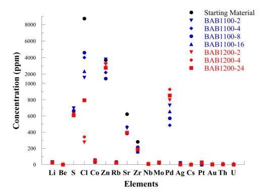
Fig. 2 - Abundance variation of minor elements in BAB samples (Rimini plant) at the two temperatures of 1100-1200°C (LA-ICP-MS analyses).
