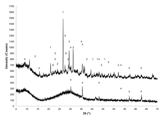
Fig. 4 - XRD scan of the untreated starting sample and of the sample after vitrification at the highest temperature and longest duration of the thermal treatment (BAP-1300-4).
