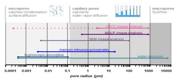
Fig. 1 - Summary of the applied analytical techniques. The resolution range of each investigation method is evidenced along with the physical process linked with the opening radius.
