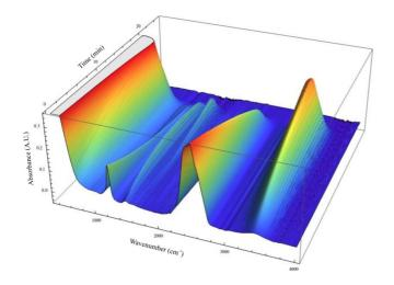
Fig. 5 - Total FTIR spectra for <sup>1</sup>H-<sup>2</sup>H exchange process.
