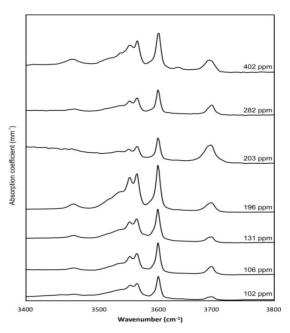
Fig. 1 - FTIR spectra of <sup>1</sup>H hydrous samples.
