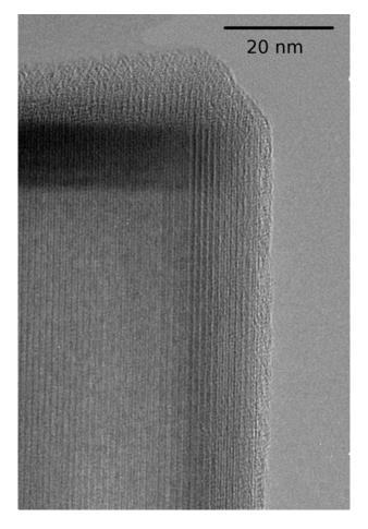
Fig. 1 - TEM image of a crocidolite fiber with probable Wadsley's defect on a side (right) and an amorphous layer of a few nanometer that rounds the whole fiber.
