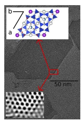
Fig. 2 - Asbestiform erionite fiber section, the high crystallinity degree is visible in the HRTEM-IFFT image. Structure and orientation are showed at the top of the image.
