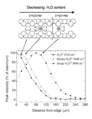
Fig. 5 - Top: schematic representation of the configuration of water molecules inside the structural channels of beryl, as the overall water content decreases. Bottom: concentration trend of selected peak for the beryl sample treated at 800 °C. Peak intensity were scaled to the maximum intensity.
