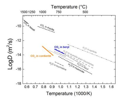
Fig. 6 - Arrhenius diagram of various diffusion coefficients D for different silicates or silicate melts for H<sub>2</sub>O and CO<sub>2</sub> (D for beryl after diffusion profiles and D for cordierite after isothermal heating experiments).
