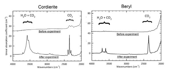
Fig. 2 - Unpolarized single-crystal spectra of a cordierite before and after treated at 900 °C and 500 MPa for 1 hour (left); unpolarized single-crystal spectra of a beryl before and after treated at 800 °C and 500 MPa for 10 hours (right).
