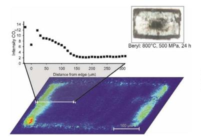
Fig. 3 - FPA image and FTIR diffusion profile of beryl treated at 800°C and 500 MPa for 24 hours.
