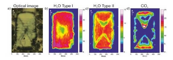
Fig. 4 - Polarized light FPA images of the beryl sample treated for four days at 800 °C, 500 MPa; a) optical image of the grain; b) E//c FTIR-FPA map of  $H_2O^{[I]}$ ; c) E//c FTIR-FPA map of  $H_2O^{[II]}$ ; (d) E⊥c FPA map of CO<sub>2</sub>. Chromatic scale is proportional to CO<sub>2</sub> content.
