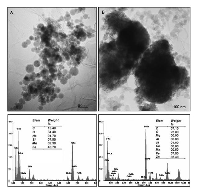
Fig. 4 - TEM images and EDX spectra of typical Fe-rich particles in atmospheric  $PM_{10}$  of Turin. (A) Agglomerate of ultrafine particles; (B) individual particles.
