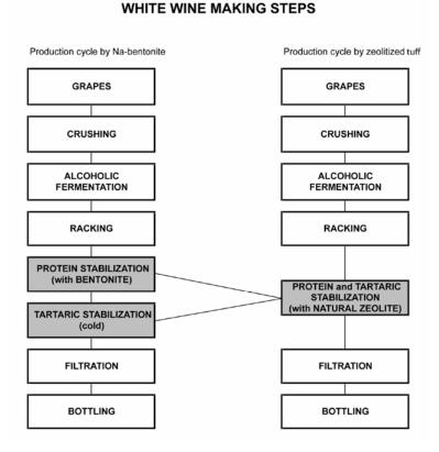
Fig. 1 - Comparison between the traditional production cycle (simplified) by using Na-bentonite (left) and the proposed one using zeolitized tuff (right) (from Mercurio *et al.*, 2010).
