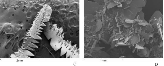
Fig. 3 - Gypsum crystals nucleated and grown in aqueous solution in the presence of DTPMP. A: concentration of  $3.5 \cdot 10^{-4}$  M; B: concentration of  $1 \cdot 10^{-4}$  M; C: concentration of  $5 \cdot 10^{-3}$  M; D: concentration of  $1 \cdot 10^{-3}$  M.
