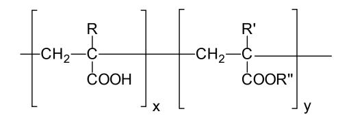
Fig. 1 - General structure of the copolymers used.
