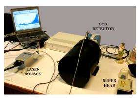
Fig. 4 – The Jobin Yvon Horiba HE532 portable spectrometer during tests at the LADIR.
