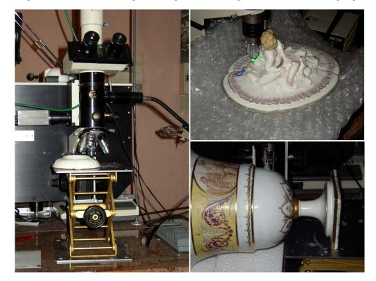
Fig. 2 – Typical experimental configuration used while acquiring micro-Raman spectra on the Sèvres Museum porcelain objects (images are not to scale).
