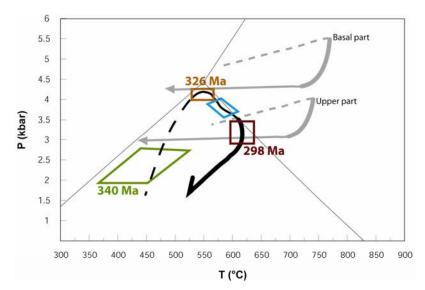
Fig. 5- P-T paths of the Hercynian crustal levels exposed in Sila: intermediate-upper crust (black lines) and lower crusts (grey lines; Graessner & Schenk, 2001). Coloured boxes represent the prograde metamorphic phases of the intermediate-upper crust. Thick segments of the P-T paths refer to the decompression P-T history directly comparable. See text for explanation.
