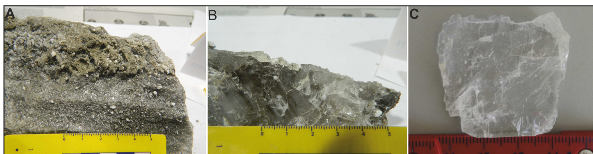
Fig. 2 - Halite samples from the Crotona basin. A) microcrystalline halite belonging to the banded facies; B) macrocrystalline halite from the white facies; C) macrocrystalline halite from the transparent facies.
