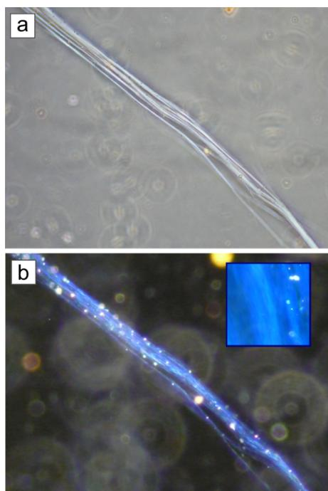
Fig. 4 - Identification of fibrous-antigorite by PLM/DS, RI 1.5680. In Phase Contrast observation fibres show a pale-blue to white colour, without halo (a), whereas they are amazing in blue indigo colour in Dark Field observation (b).
