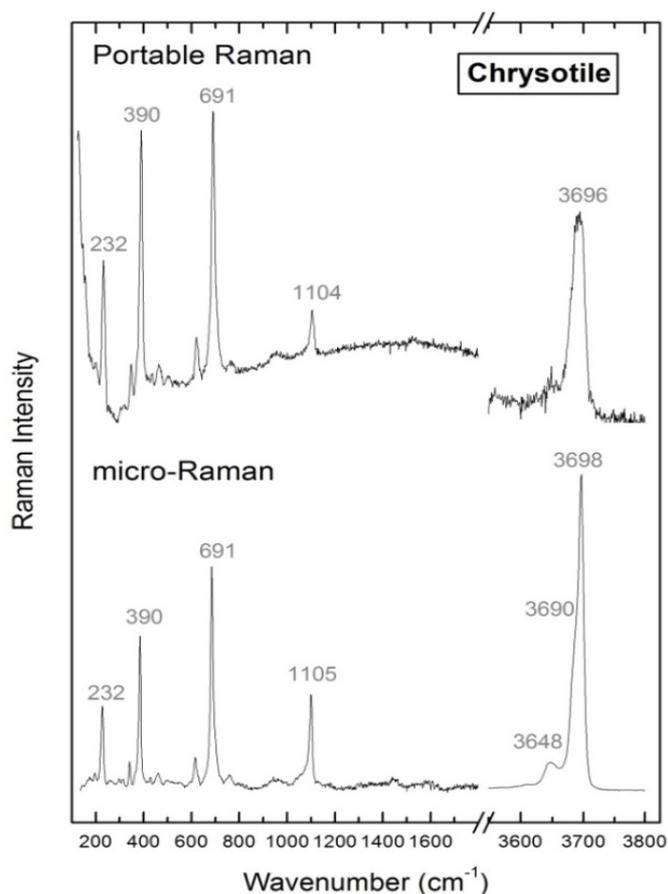
Fig. 5 - Comparison of spectra recorded with a micro-Raman spectrometer (473.1 nm laser) and a portable Raman device (532 nm laser).
