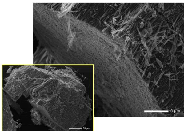
Fig. 3 - SEM images of compact bundle of parallel fibrils of chrysotile.
