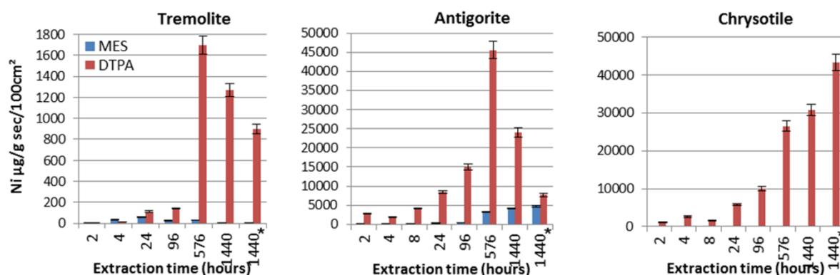
Fig. 7 - Ni concentration in the supernatant as a function of time for leaching experiments with two solutions MES and DTPA. \* for experiments conducted with several asbestos-fragments leading possible mechanical effect on alteration during shaking.
