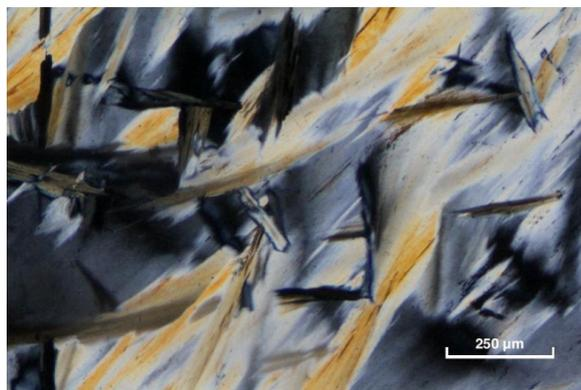
Fig. 2 - PLM cross-polarizing image showing an unusual and potential new type of texture, characterized by star and fan formed aggregates. Finely intergrowth of fibrous antigorite and chrysotile fibres at the micro-scale.
