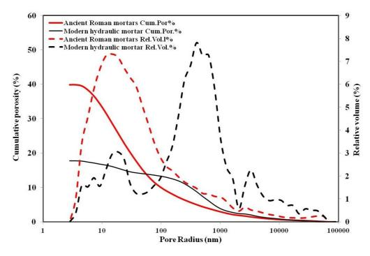
Fig. 4 - Cumulative and relative pore size distribution in Roman mortars compared with SHM (Standard Hysdraulic Mortar).
