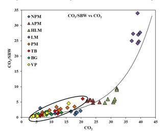
Fig. 3 - CO<sub>2</sub>/SBW vs. CO<sub>2</sub> diagram, comparing data from analyzed Roman mortars (black circle) and from Moropoulou *et al.*, 2005. (NPM: natural pozzolanic mortars; APM: artificial pozzolanic mortars; HLM: Hydraulic lime mortars; LM: lime mortars; PM: Piscina Mirabilis; TB: Terme di Baia; BG: Villa del Capo; VP: Villa del Pezzolo).
