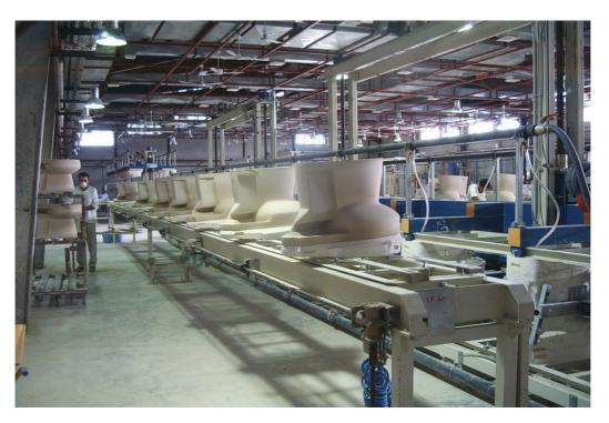
Fig. 2 - Casting sanitaryware industrial process.
