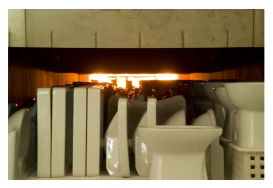
Fig. 3 - Ceramic kiln for sanitaryware.
