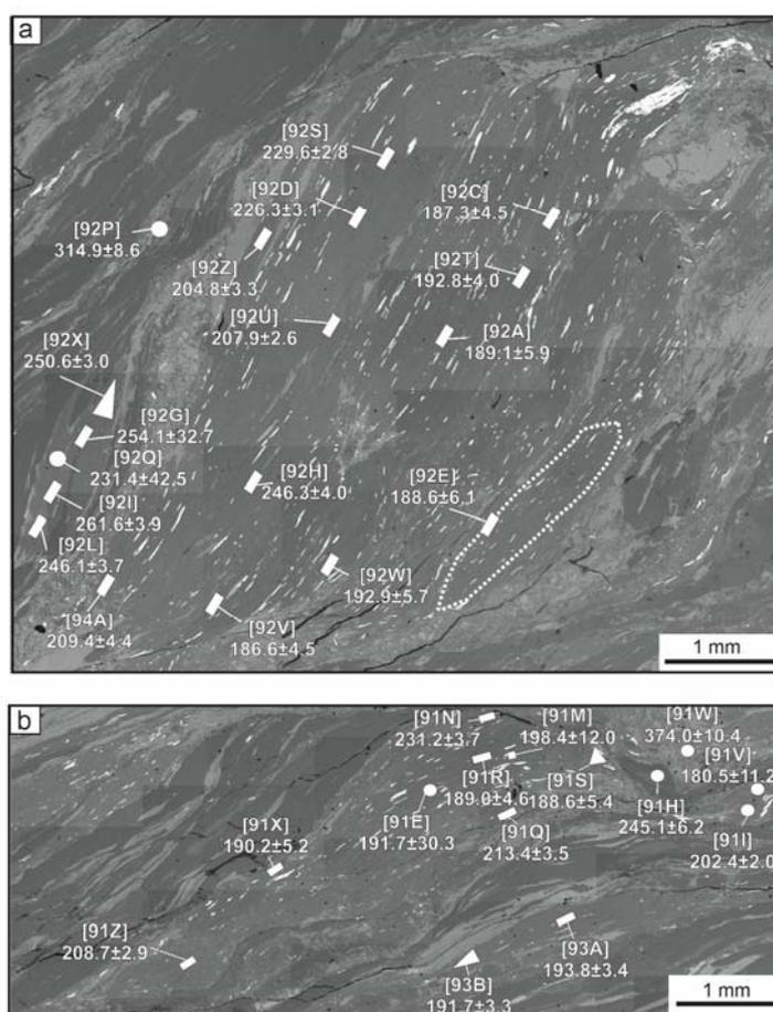
Fig. 3 - BSE images of chip A (a) and chip B (b) with the location of the step-heating area (dotted line), the IR laser spots (circles) and UV laser pits (squares, rectangles and triangles) in the mylonites from the Cerreto Pass. The corresponding ages are reported with the  $2\sigma$  analytical uncertainty.
