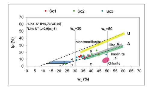
Fig. 3 - Casagrande chart: 1) Inorganic silts, low compressibility; 2) Inorganic silts and organic clays, medium compressibility; 3) Inorganic silts and organic clays high compressibility; 4) Inorganic clays, low plasticity; 5) Inorganic clays, medium plasticity; 6) Inorganic clays, high plasticity.
