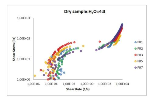
Fig. 4 - Rheological analysis diagram considering the amount of water lower than the amount of specimens, performed on samples collected from the sliding zone.
