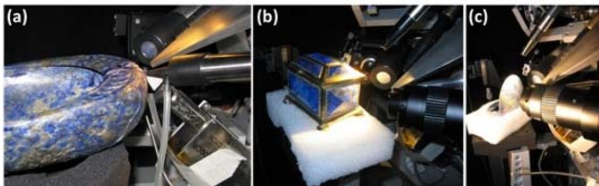
Fig. 5 - a) Oval Bowl, b) Small case, and c) Oval panel of the “Collezione Medicea” positioned for the measurements at the external micro-beam of LABEC.
