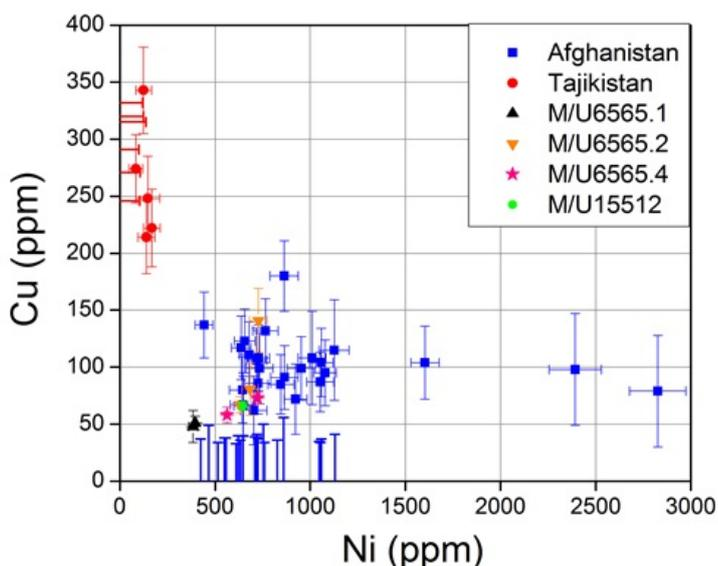
Fig. 6 - Cu vs. Ni contents in pyrite from  $\mu$ -PIXE measurements. The individual errors associated to each measurement are plotted, whereas the values below the LOD are represented by a bar indicating the LOD value for each measurement. In different colours, the experimental data related to the “Savoy Collection” artefacts overlying to the data cluster of the Afghan samples.
