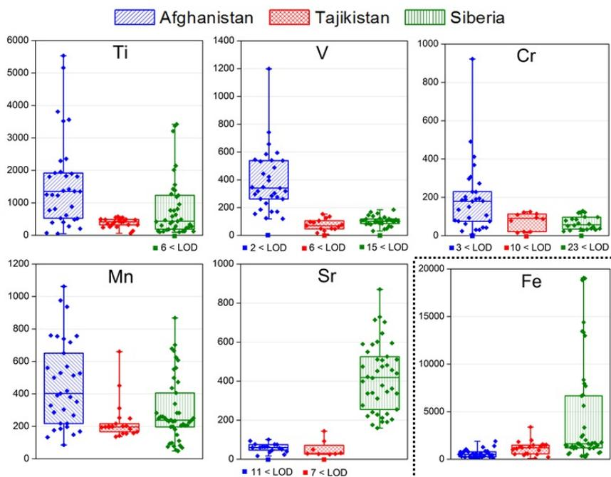
Fig. 1 - Trace and minor (Fe) elements content in diopside (expressed in ppm). Each point is an individual  $\mu$ -PIXE measurement and the box charts represent the dispersion of the experimental points: the median and the two percentile values 0.25 and 0.75. The bars join the minimum and maximum values and the symbols in correspondence to zero value represent the number of measurements below the LOD (as specified at the bottom of each graph).
