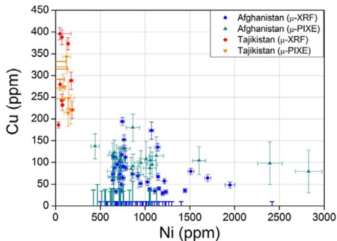
Fig. 3 - Binary graph Cu vs. Ni, the individual errors associated to each measurement carried out by means of both techniques are represented: the statistical error and the GUPIXWIN output (fit error) were respectively considered for  $\mu$ -XRF and  $\mu$ -PIXE measurements.
