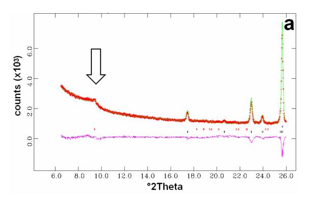
Fig. 3 - Graphical output (observed, calculated and curve of the differences) of the Rietveld refinement for the quantitative phase analysis of antigorite heated at 800  $^{\circ}$ C.
