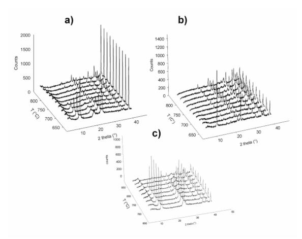
Fig. 2 - Dynamic XRPD experiments on antigorite (a), lizardite (b) and chrysotile (c).
