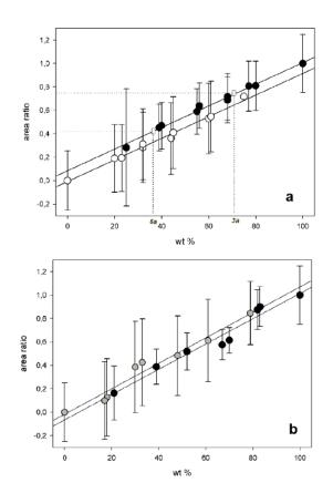
Fig. 1 - Correlation curves between total area ratio and chrysotile amount (wt.%) for Lz + Ctl (a) and Atg + Ctl (b) samples; standard error associated with each measure is represented by error bars. Legend: black dots = Lz; gray dots = Atg; white dots = Ctl; white squares = the two investigated unknown samples 3a and 5a.
