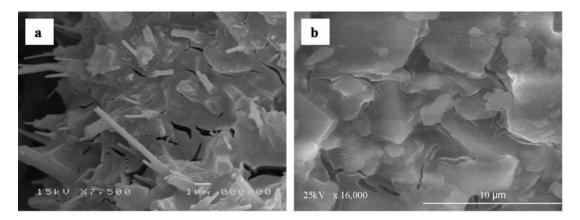
Fig 1 - SEM microphotographs of consolidant (ES) distribution on NYT (a) and VS (b) surface.
