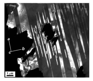
Fig. 2 - A typical texture of amphibole lamellae (white contrast) in the clinopyroxene (black matrix). The both phases share the (010) planes in the same direction. Dark field TEM image with  $\mathbf{g} = 5\overline{10}$  (in the clino-amphibole diffraction).
