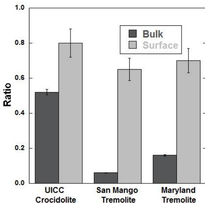
Fig. 1 - Comparison of  $\text{Fe}^{3+}/\text{Fe}_{\text{tot}}$  atomic ratios between bulk (Mössbauer results) and surfaces (XPS results) of asbestos samples.
