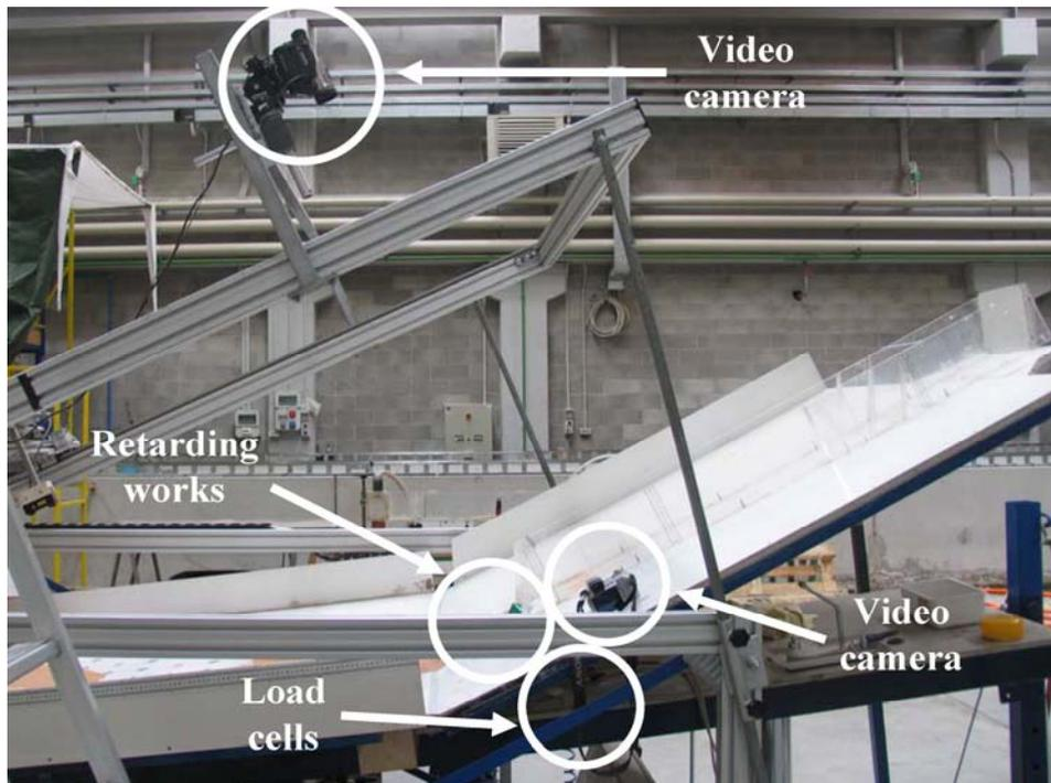
Fig. 4 - The experimental chute with the instrumentation. The channel width was 0.20 m, its length was 1.50 m and its slope inclination was 24°-27°-30°. The width of the downstream plane was 1.50 m, its length 1.50 m and its slope inclination was 7° (Laboratory of the University of Trento, Italy).
