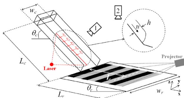
Fig. 2 - Sketch of the experimental set-up and instrumentation. The channel width ( $w_c$ ) was 0.30 m, its length ( $L_c$ ) was 1.50 m and its slope inclination ( $\theta_c$ ) was 35°. The width of the downstream plane ( $w_r$ ) was 1.20 m, its length ( $L_r$ ) 2.50 m and its slope inclination ( $\theta_r$ ) was 6° (Laboratory of the Cemagref de Grenoble, France).
