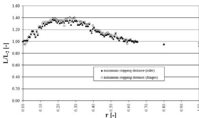
Fig. 3 - Stopping distance of the deposit ( $L$ ) normalized by the stopping distance of the deposit ( $L_2$ ) obtained with the large grains of diameter only versus the mass ratio in fine particles ( $r$ ). Results from the fringes projection technique (white circles) as well as from the direct measurements with a ruler (black triangles) are shown.
