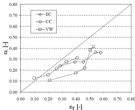
Fig. 5 - Relationship between mean values of cross-sectional efficiency ( $\epsilon_T$ ) and longitudinal efficiency ( $\epsilon_L$ ) for the various type of retarding structures systems for the three different type of structures.
