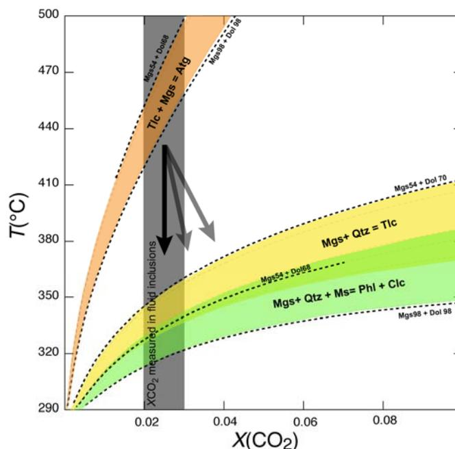
Fig. 2 - *T-P-X(CO<sub>2</sub>)* projection. Coloured areas outline the location of reactions as a function of magnesite compositional range. The grey bar corresponds to calculated X(CO<sub>2</sub>). The arrows point out the possible trajectories for the fluid path.
