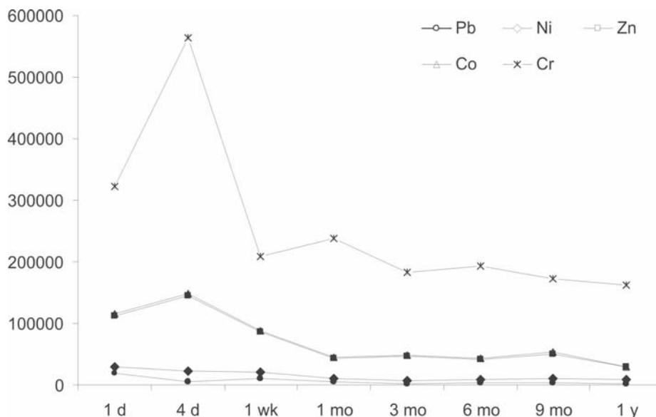
Fig. 1 - Heavy metal extraction with single-step procedure in experiments in laboratory.
