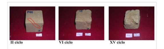
Fig. 3 - Loss of material around "skolithos" during II-VI-XV salt crystallization cycle.
