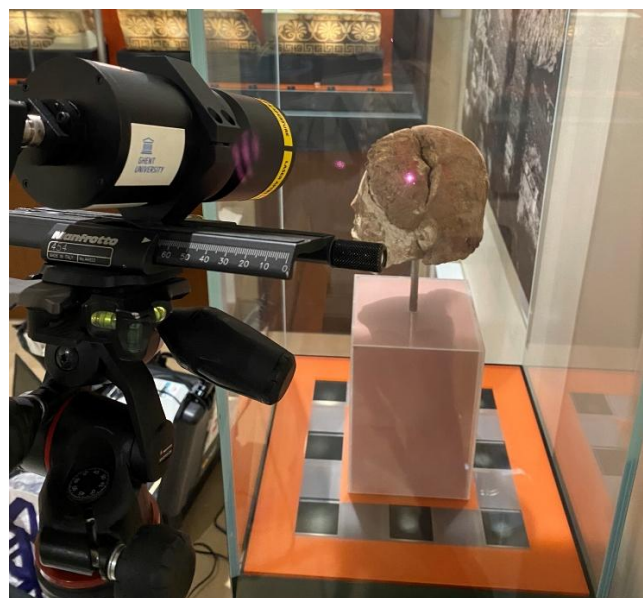
Figure 1 Image of the in situ Raman measurement in action.
