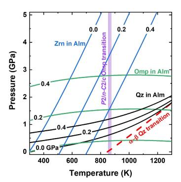
**Figure 6** Calculated isomekes for quartz ( $\Omega z$ ), zircon (Zrn) and omphacite (Omp) inclusion in an almandine (Alm) host. The  $\alpha$ - $\beta$  quartz and the P2/n-C2/c omphacite transitions are also represented. Modified after Baratelli et al. (2024).
