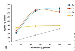
Figure 1 a) REE fraction drawn from solution as a function of the solid/liquid ratio. b) Amount of REE incorporated in the zeolite as a function of the solid/liquid ratio.
