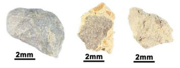
Figure 4 Recycled aggregates with variable amounts of LCP (reproduced from Bisciotti et al., 2024).
