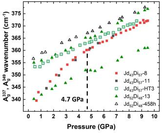
**Figure 4** Pressure dependence of the Raman peaks in the range 335-375 cm<sup>-1</sup>. For sample  $\mathrm{Jd}_{43}\mathrm{Di}_{57}$  only one peak at 337 cm<sup>-1</sup> was detected experimentally, with an anomalous behaviour near 4.7 GPa in the ordered crystals. For sample  $\mathrm{Jd}_{52}\mathrm{Di}_{48}$  two peaks were resolved, but an anomaly is still visible. Filled symbols are related to ordered omphacites, while open symbols to disordered ones.
