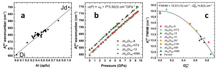
Figure 3 a) Chemical composition and b) pressure dependence of the wavenumber of the peak at 681 cm<sup>-1</sup>. The wavenumber increases linearly with P, but is also influenced by omphacite composition. c) The cation order affects the FWHM of the peak at 681 cm<sup>-1</sup>, with a parabolic dependence. b) and c) are modified after Baratelli et al. (2025a). Filled symbols are related to ordered omphacites, while open symbols to disordered ones.
