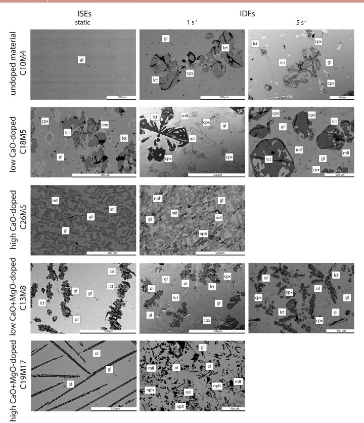
Figure 6 BSE photomicrographs illustrating the phase assemblage and textural features resulting from ISEs and IDEs. Gl: glass, Ol: olivine, Cpx: clinopyroxene, Lct: leucite, Nph: nepheline, Mll: melilite.
