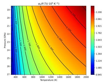
**Figure 3** Contour plot of ab initio volume thermal expansivity of  $Mg_2SiO_4$  ringwoodite at mantle transition zone conditions.
