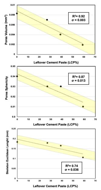
Figure 9 Comparison of LCP% and concrete microstructure.
