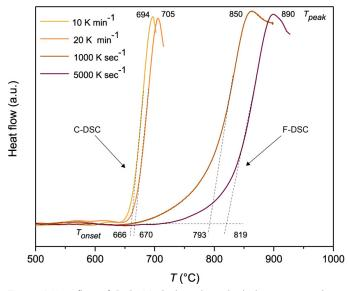
**Figure 4** Heat flow of CaO+MgO-doped residual glass measured as a function of temperature using conventional (C-DSC) and Flash (F-DSC) differential scanning calorimetry. Dashed lines correspond to the second upscan during measurements performed at 10 and 20 K min<sup>-1</sup> and at 1000 and 5000 K s<sup>-1</sup> using the rate-matching method (Di Genova et al., 2020).
