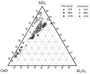
**Figure 1** Triplot for the XRF major oxides composition (reproduced from Bisciotti et al., 2025).
