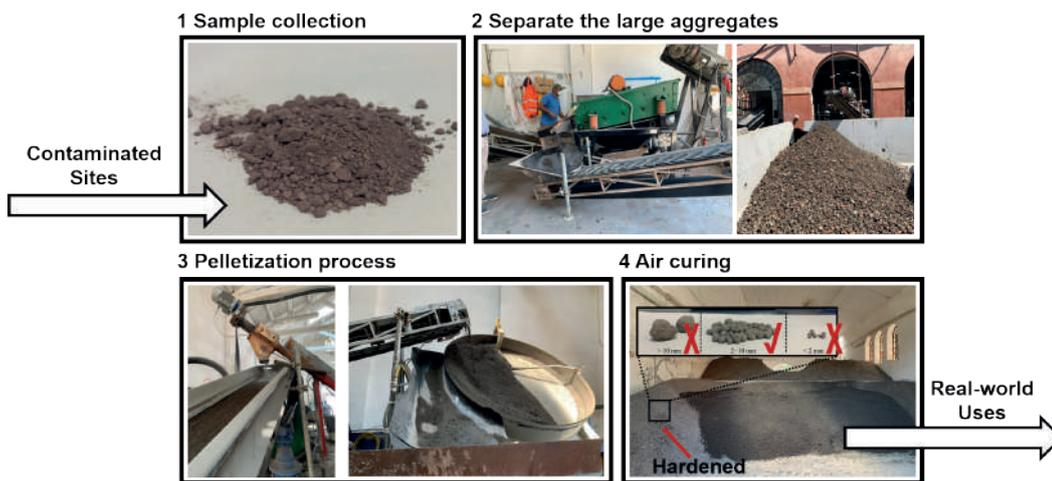
Figure 2 HPSS® process framework.
