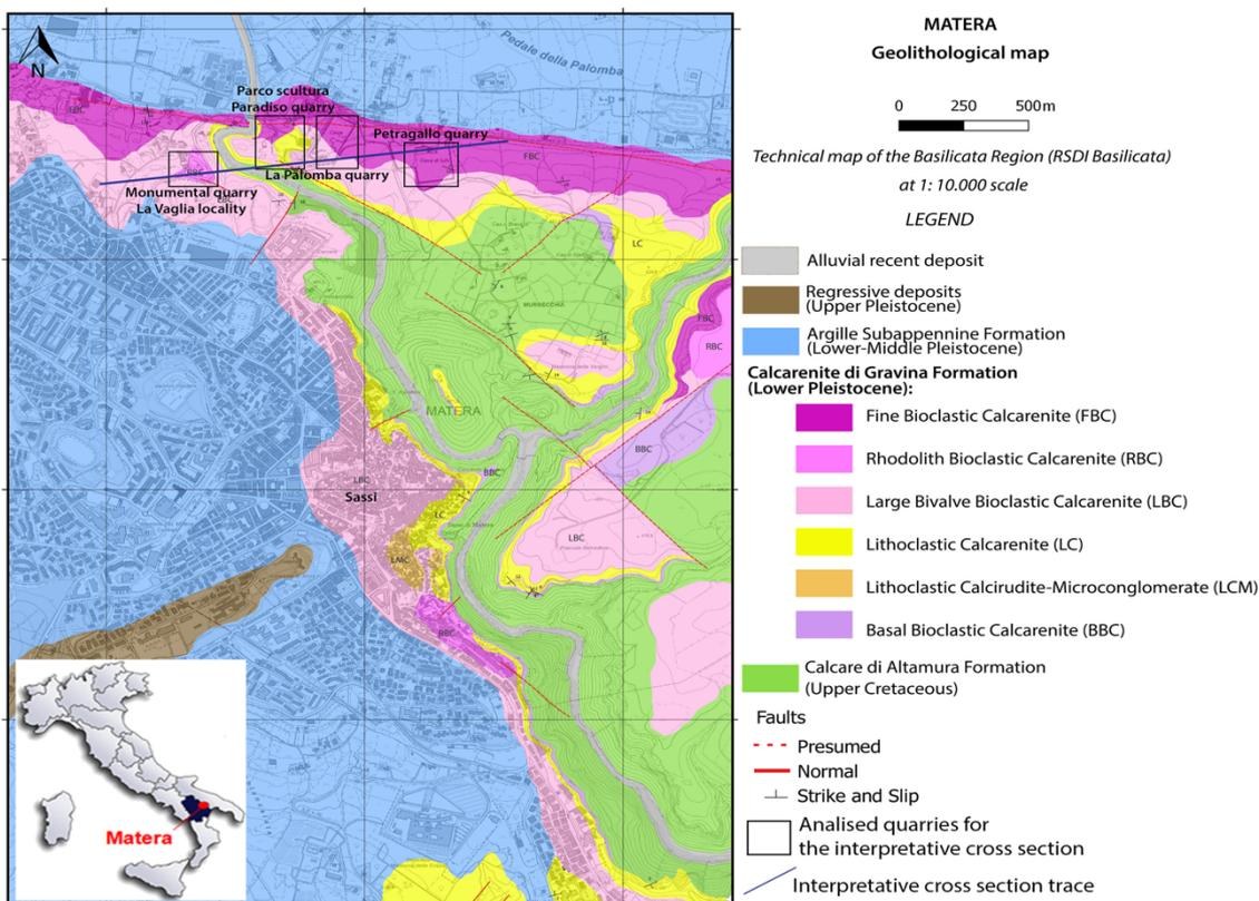
Fig. 2 - Geolithological map based on the technical map of the Basilicata Region (RSDI Basilicata) at 1: 5.000 scale.
