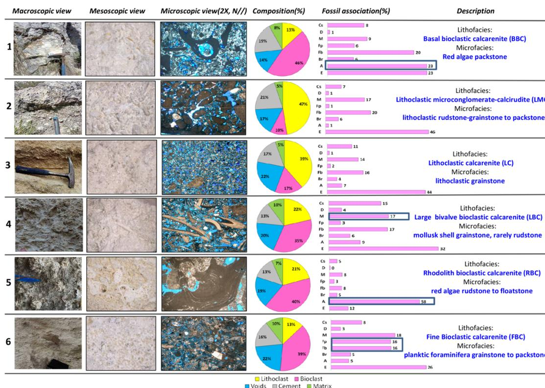
Fig. 1 - Summary of the six calcarenite lithofacies and microfacies identified on the basis of field and OM observation as well as quantitative measurement made by point counting of the main components (cake diagram) and of the bioclast types (bar histogram). Bioclast are: echinoderm (E), red algae (A), benthic foraminifera (Fb) planktonic foraminifera (Fp), mollusk shells (M), unidentified calcitic shell fragments (Cs), bryozoan (Br), ditrupa tubiphytes (D).
