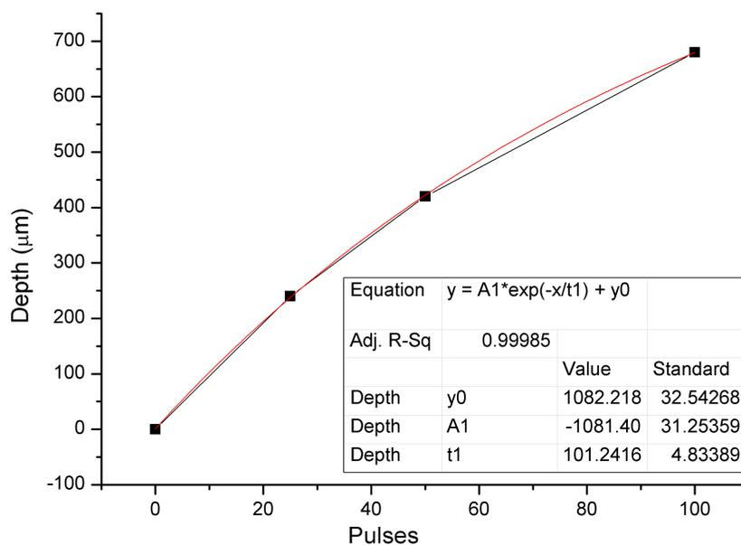
Fig. 3 - Depth of craters ( $\mu\text{m}$ ) vs. number of laser pulses. The depth of craters follow approximatively an exponential curve.
