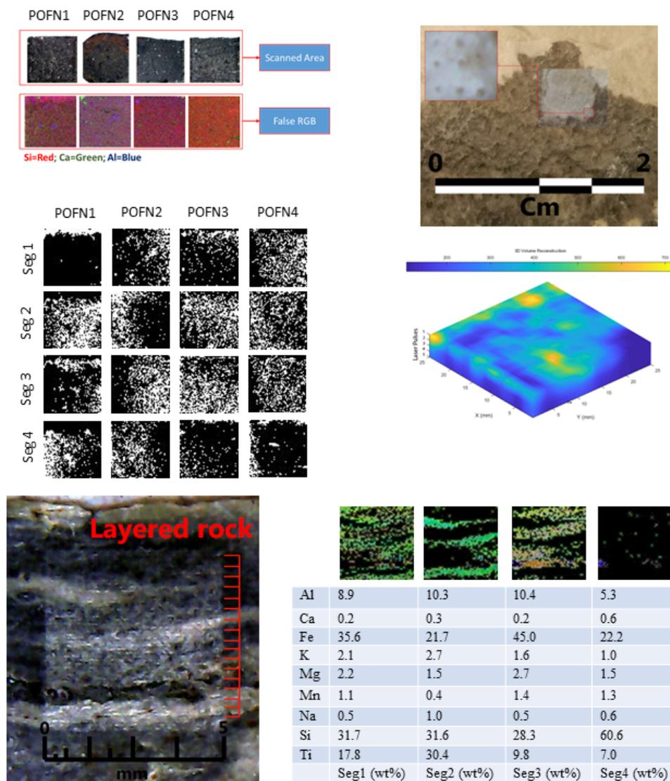
Fig. 4 - Some examples of the capability of the system: elemental maps, false color map (combining different maps), Artificial Intelligence segmentation of the map features and 3D reconstruction of the ablated surfaces.
