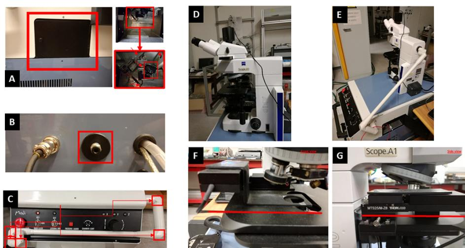
Fig. 1 - The different part of the MODÌ instrument. A) Main analysis chamber with some details; B) backpanel with airflow nozzle; C) external articulated arm with the indication of reflecting mirror positioning; D) the microscope with digital camera; E) the microscope attached to the instrument by mean of the articulated arm; F) scanning system X axis; G) scanning system Y axis.
