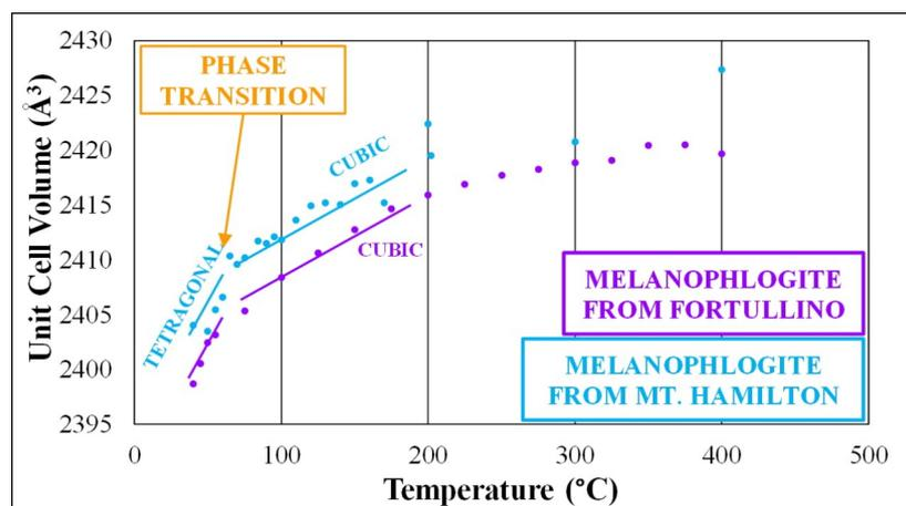
Fig. 1 - HT-XRPD on melanophlogite from Fortullino, from room temperature up to 400 °C, compared with results for melanophlogite from Mt. Hamilton (Nakagawa *et al.*, 2005).
