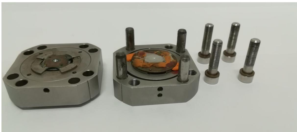
Fig. 2 - Components of an ETH-type diamond anvil cell with the four screws used to load to the diamonds
