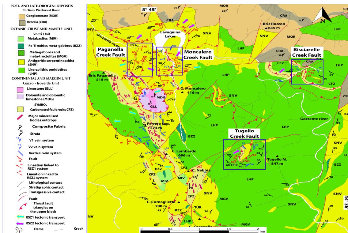
Fig. 1 - Structural sketch of the Lavagnina Lakes Area, redrawn with updates and georeferenced with Qgis open source software (modified after Spagnolo *et al.*, 2007). In this sketch, the four structures analysed in detail are highlighted with the blue squares.
