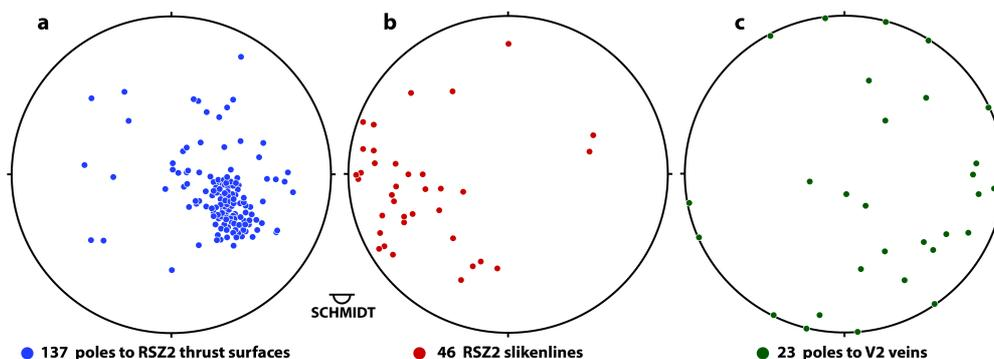
Fig. 3 - Stereographic projections. (a) Poles to RSZ2 thrust surfaces (137 points). (b) Slickenlines (46 points). (c) Poles to V2 veins (23 points). The data are from the field survey for this work.
