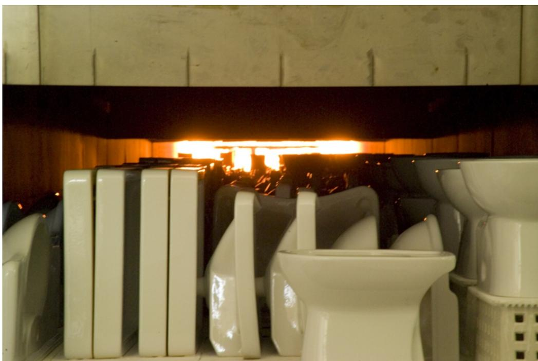
Fig. 3 - Ceramic kiln for sanitaryware.
