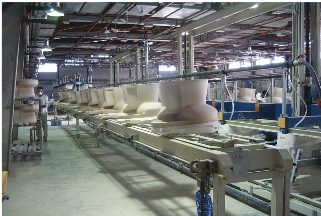
Fig. 2 - Casting sanitaryware industrial process.
