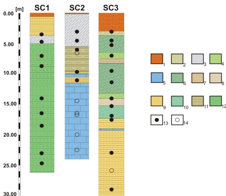
Fig. 1 - Stratigraphic sequences of the studied area: 1) top soil; 2) greyish-green silty shales; 3) shales; 4) greenish silty shales; 5) calcarenitic sandstones; 6) greyish silty shales; 7) brownish silty shales ; 8) silty sands; 9) sandstones; 10) bluish-gray silty shales; 11) greyish clayey silts; 12) marly shales with calcareous clasts; 13) samples selected for mineralogical and geotechnical analyses; 14) samples selected for mineralogical analyses.
