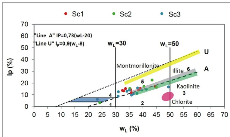
Fig. 3 - Casagrande chart: 1) Inorganic silts, low compressibility; 2) Inorganic silts and organic clays, medium compressibility; 3) Inorganic silts and organic clays high compressibility; 4) Inorganic clays, low plasticity; 5) Inorganic clays, medium plasticity; 6) Inorganic clays, high plasticity.
