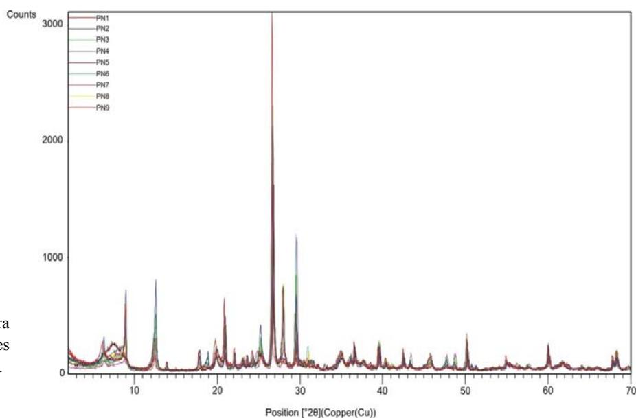
Fig. 2 - XRPD spectra representative of samples collected from the crown zone.
