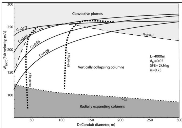
Fig. 3 - Regime diagram showing the stability fields of the three main eruptive regimes, by fixing the parameters, shown on the right, and varying the average particles concentration  $C$  (black lines). The thick dashed lines represent eruption rates, ER, of  $10^7$  and  $10^8 \text{ kg s}^{-1}$ , respectively.
