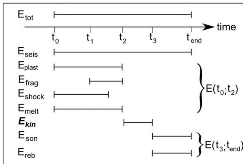
Fig. 1 - Chronology of energy dissipation during a brittle fragmentation experiment.  $E_{kin}$  is the wanted quantity and is highlighted. It is the only energy term dissipated in the time interval  $[t_2; t_3]$ ; thus, as the total energy  $E_{tot}$  is known and by determining  $E(t_0; t_2)$  and  $E(t_3; t_{end})$ , it can be readily obtained by subtraction.
