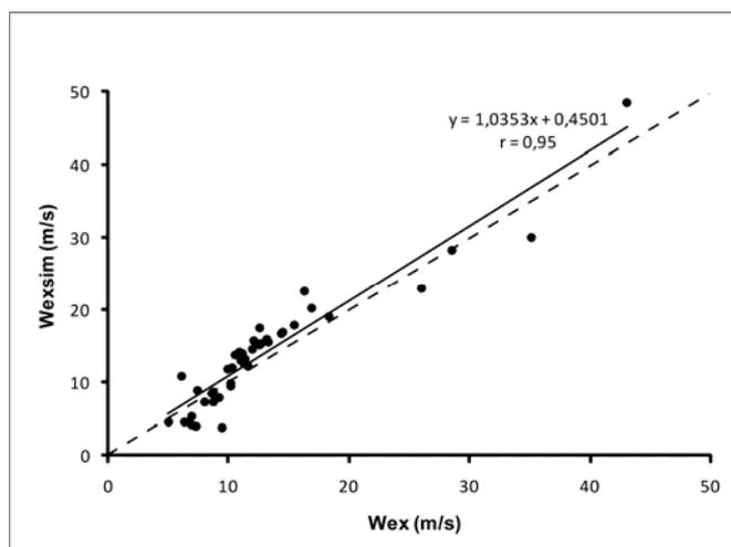
Fig. 4 - Simulated vs. measured exit velocity for all the experiments. The dashed line represents the perfect agreement, the solid line is the linear regression with the equation and the correlation coefficient  $r$  in the inset.
