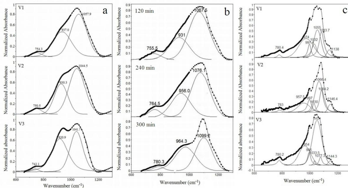
Fig. 1 - a) Fit (thick line) of the unaltered V1, V2 and V3 FT-IR spectra (points) through decomposition (thin lines) into vibrational contributions; b) Fit (thick line) of the leached V3 samples FT-IR spectra (points) through decomposition (thin lines) into vibrational contributions, over the leaching time; c) Fit (thick line) of the V1, V2 and V3 FT-IR spectra (points) through decomposition (thin lines) into vibrational contributions, after dissolution experiments.
