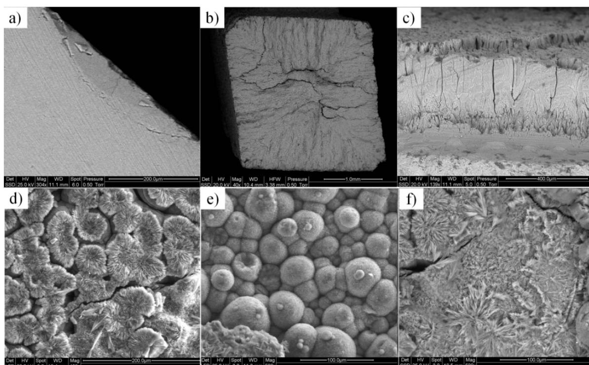
Fig. 3 - a) Backscattered electron (BSE) image of the cross section of a V1 sample aged for 2 weeks in  $H_2SO_4$ ; b) BSE image of the cross section of a V3 sample aged for 6 hours in  $H_2SO_4$  where the alteration extends to the whole volume; c) BSE image of cracks crossing the alteration layer of the V1 sample after the dissolution experiments; d, f) Secondary Electron (SE) e) BSE images of crystallized phases on the V2 and V3 surfaces.
