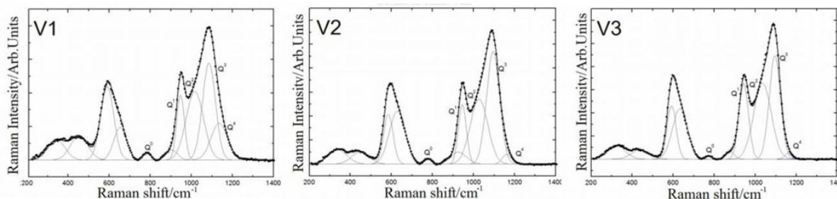
Fig. 2 - Fit (thick line) to the V1, V2 and V3 Raman spectra (points) through de-composition (thin lines) into the  $Q^n$  contributions.
