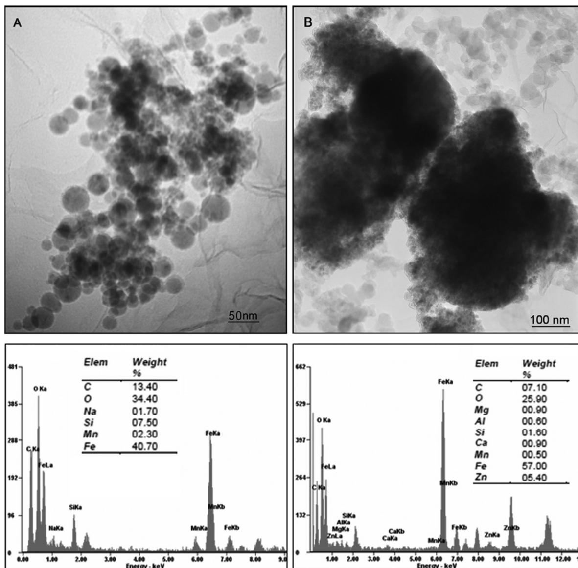
Fig. 4 - TEM images and EDX spectra of typical Fe-rich particles in atmospheric PM<sub>10</sub> of Turin. (A) Agglomerate of ultrafine particles; (B) individual particles.
