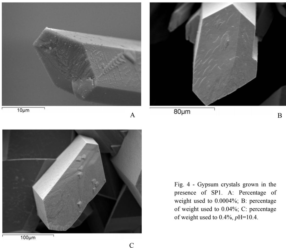
Fig. 4 - Gypsum crystals grown in the presence of SP1. A: Percentage of weight used to 0.0004%; B: percentage of weight used to 0.04%; C: percentage of weight used to 0.4%, *pH*=10.4.
