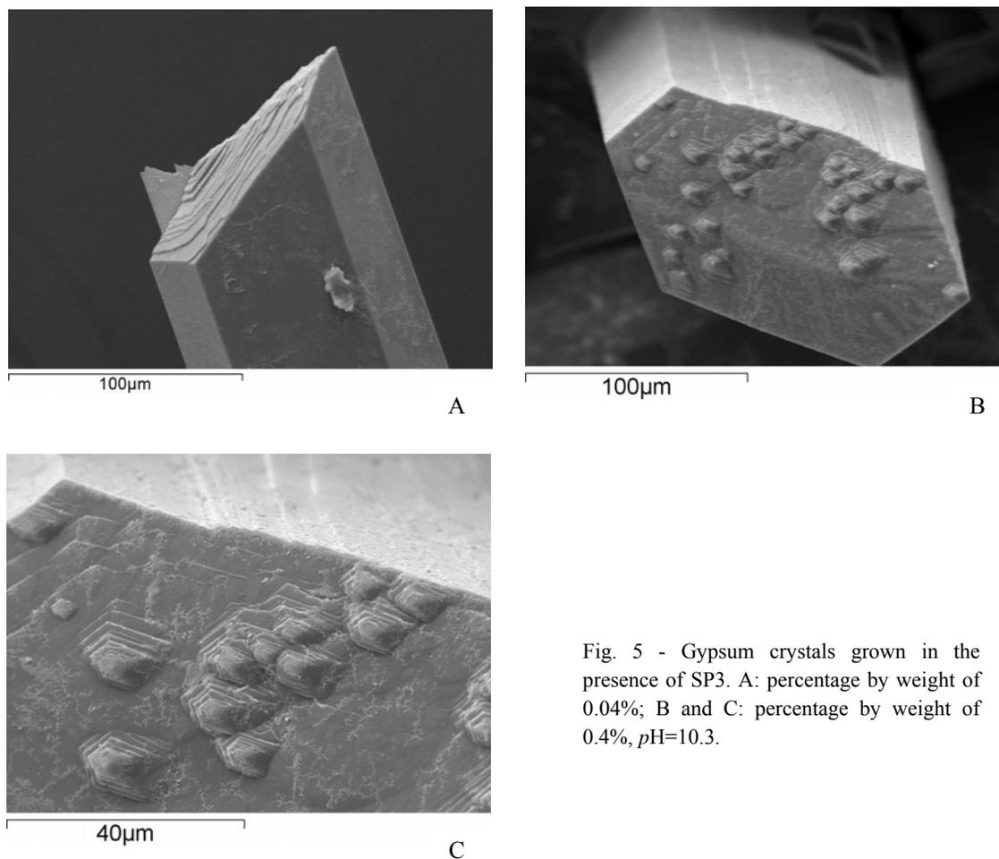
Fig. 5 - Gypsum crystals grown in the presence of SP3. A: percentage by weight of 0.04%; B and C: percentage by weight of 0.4%,  $pH=10.3$ .
