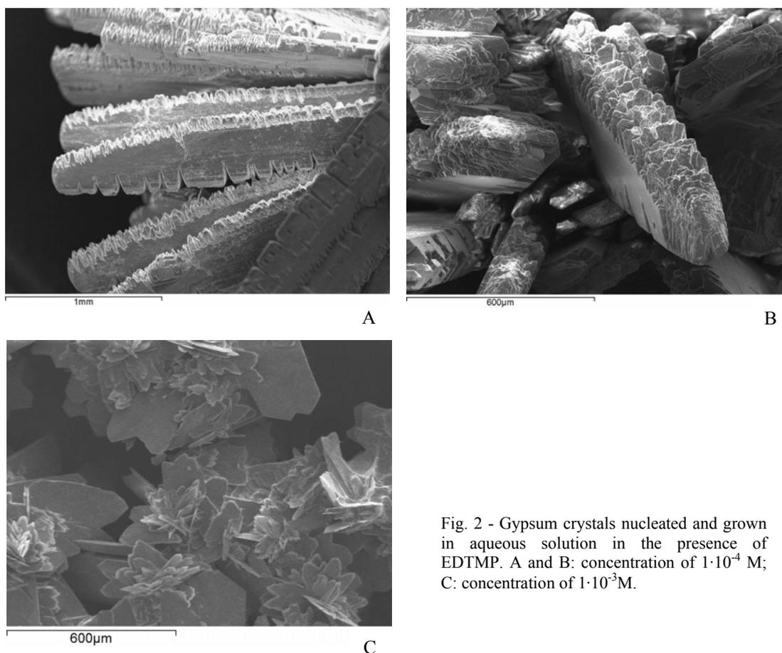
Fig. 2 - Gypsum crystals nucleated and grown in aqueous solution in the presence of EDTMP. A and B: concentration of  $1 \cdot 10^{-4}$  M; C: concentration of  $1 \cdot 10^{-3}$  M.
