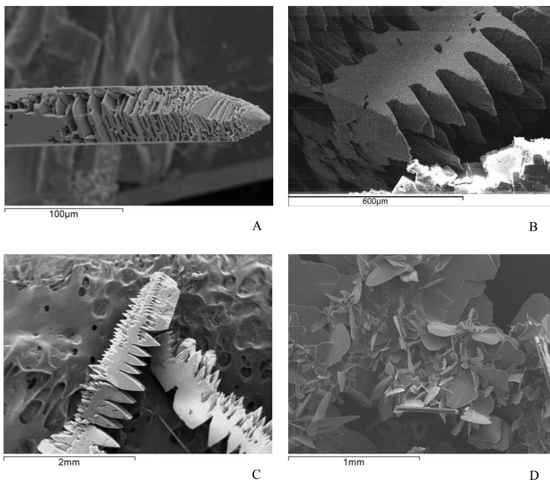
Fig. 3 - Gypsum crystals nucleated and grown in aqueous solution in the presence of DTPMP. A: concentration of  $3.5 \cdot 10^{-4}$  M; B: concentration of  $1 \cdot 10^{-4}$  M; C: concentration of  $5 \cdot 10^{-3}$  M; D: concentration of  $1 \cdot 10^{-3}$  M.
