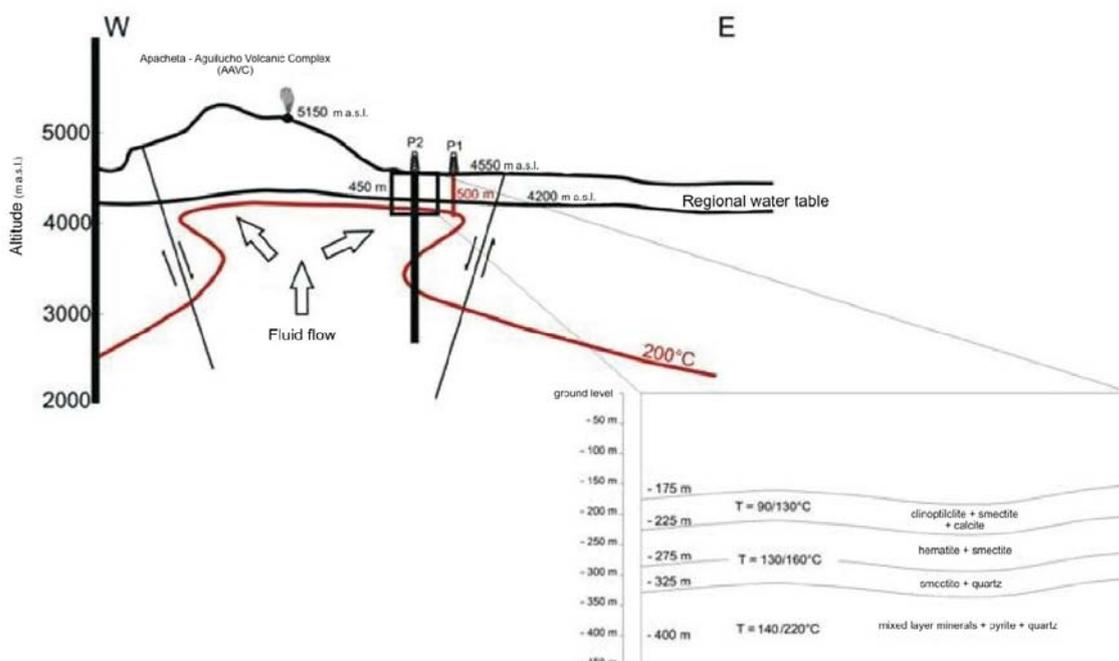
Fig. 6 - Cross section of the AAVC geothermal area coupling hydrogeological and geophysical (MT) data from Urzua *et al.* (2002) and hydrothermal mineral zonation (present work).
