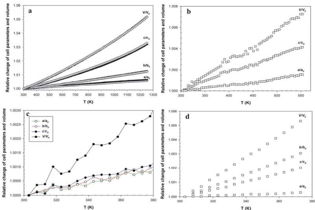
Fig. 2 – Relative expansion of lattice parameters and volume in phases of  $\text{CaSO}_4\text{-H}_2\text{O}$  system (*a* β-anhydrite, *b* γ-anhydrite, *c* bassanite, and *d* gypsum).
