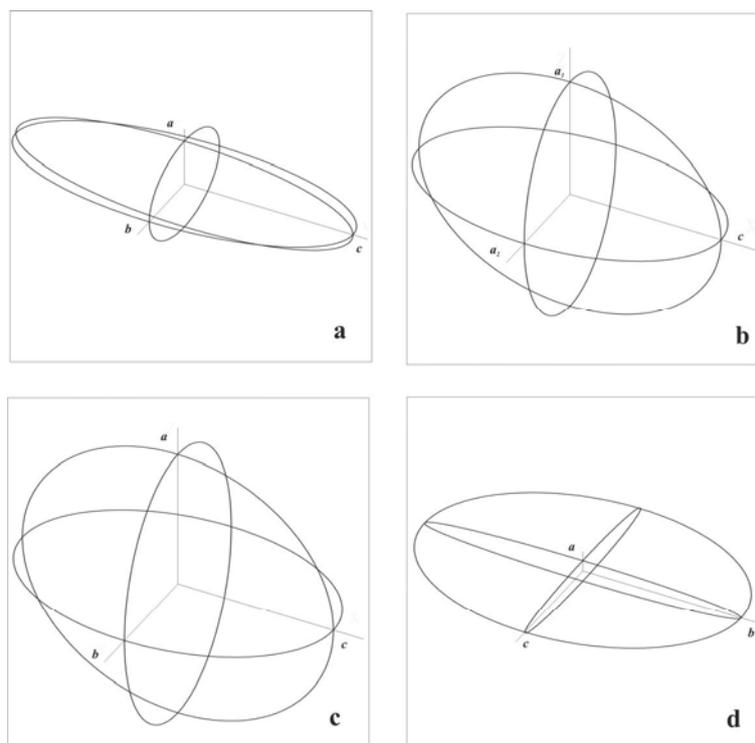
Fig. 3 – Unit strain ellipsoid (Ohashi, 1972) of the  $\text{CaSO}_4\text{-H}_2\text{O}$  system (**a**  $\beta$ -anhydrite, **b**  $\gamma$ -anhydrite, **c** bassanite, and **d** gypsum).
