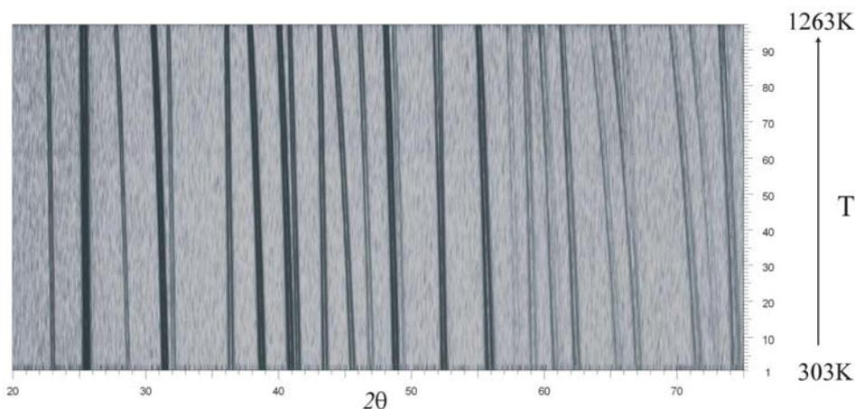
Fig. 1 – Magnified view (20-75° 2θ) of the complete data set of the thermal expansion of β-anhydrite shown as a pseudo Guinier plot.
