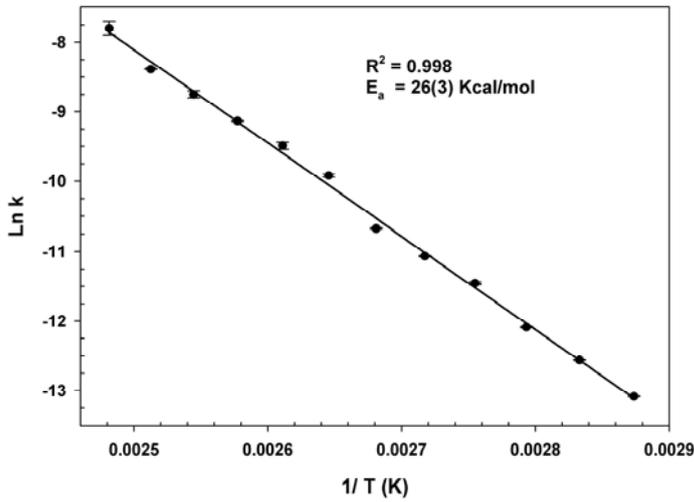
Fig. 5 – Arrhenius  $\ln k$  vs.  $1/T$  plot for the gypsum  $\rightarrow$  bassanite conversion.
