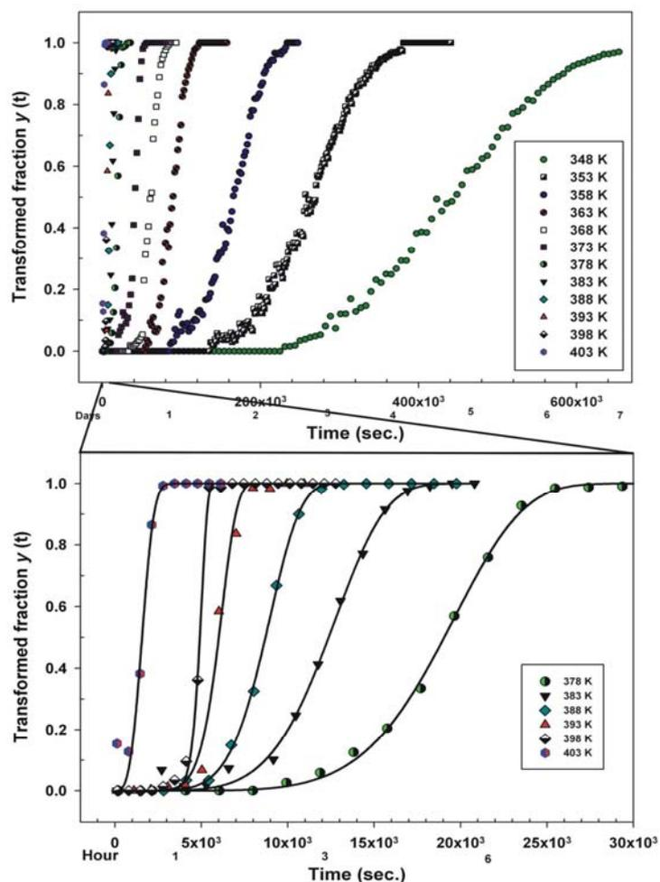
Fig. 4 – Curves  $\alpha$  vs. time of dehydration of gypsum in the temperature range 348-403 K with a  $\Delta$  of 5 K.
