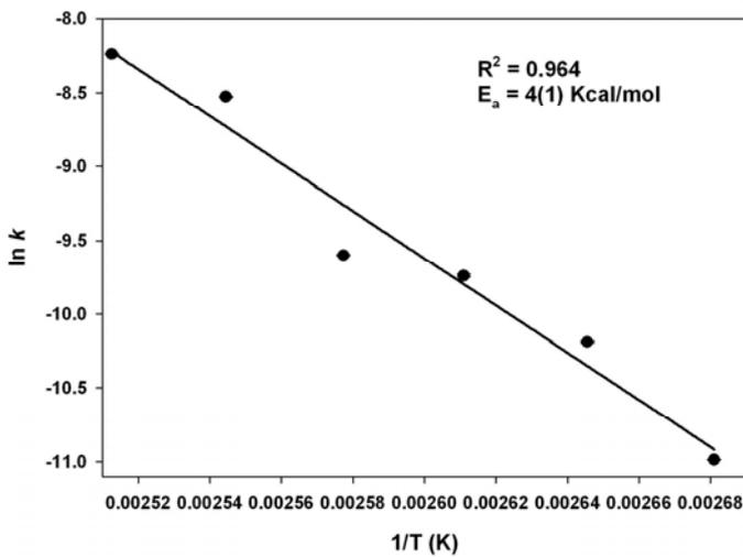
Fig. 7 – Arrhenius  $\ln k$  vs.  $1/T$  plot for the bassanite  $\rightarrow$   $\gamma$ -anhydrite conversion.
