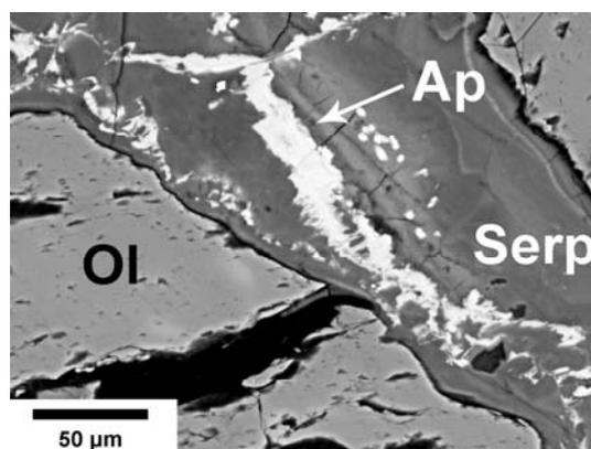
Fig. 3 - Back-scattering image showing a (Na,S)-rich fluorapatite (Ap) veinlet in serpentine (Serp).
