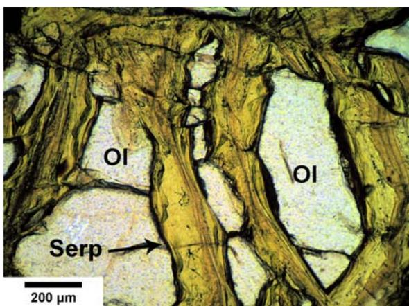
Fig. 2 - Composite structure of serpentine veins (Serp), inside olivine grains (Ol).
