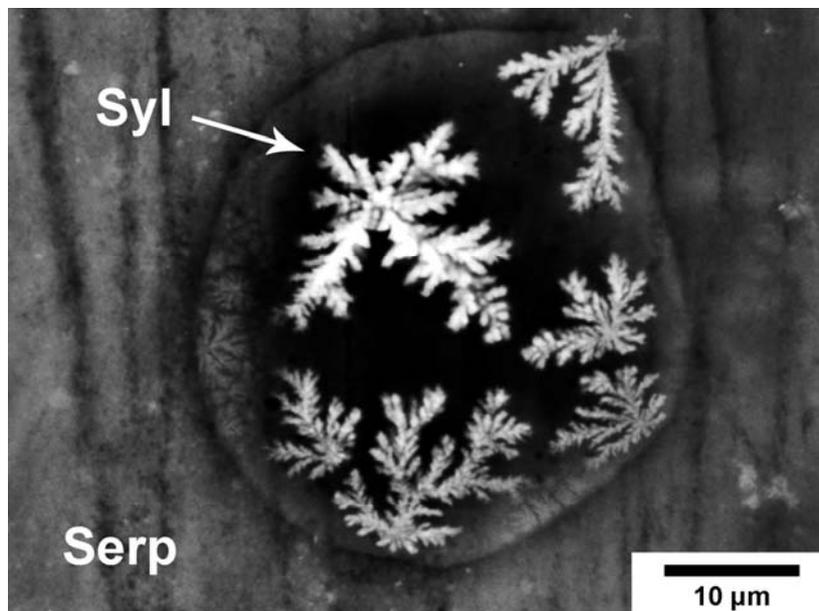
Fig. 4 - Back-scattering image of a dendritic aggregate of Na-sylvite (Syl) in a fluid inclusion in serpentine.
