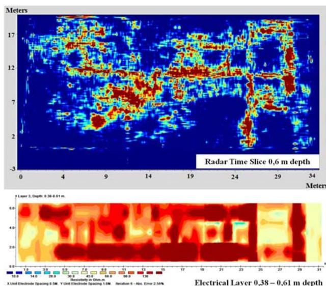
Fig. 3 - Visual comparison between the different methodologies used for buried structures reconstruction.
