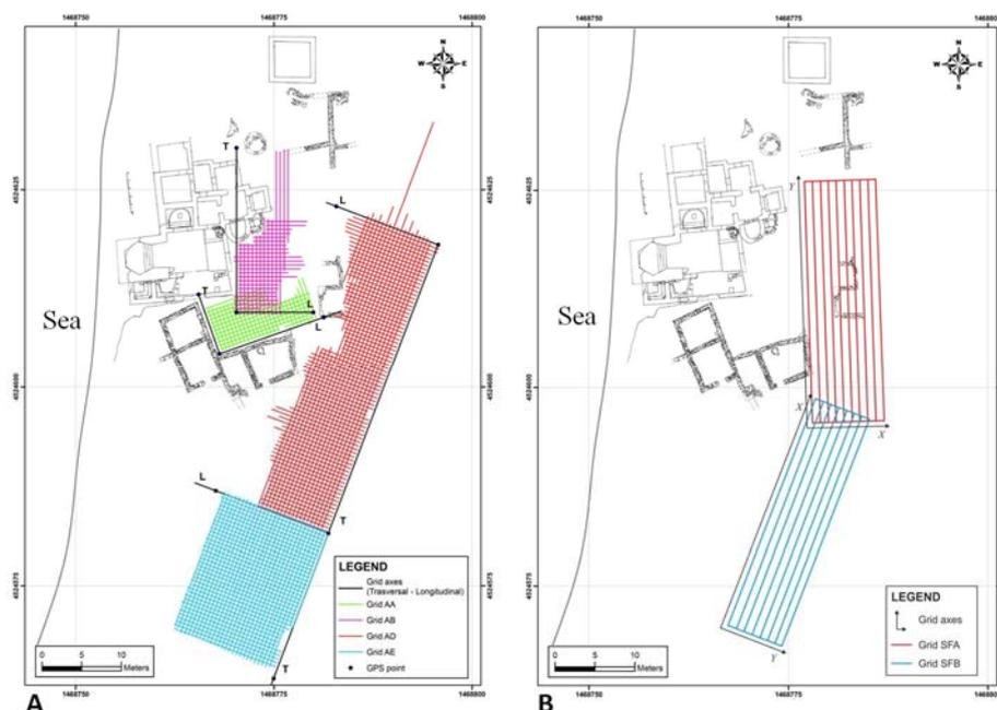
Fig. 4 - A) Site plan including GPR surveys location. B) Site plan including electrical resistivity surveys position.
