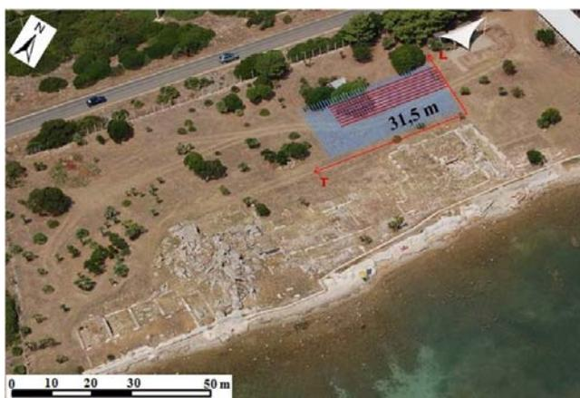
Fig. 2 - Survey location. The red lines show the electrical surveys, the blue lines show the GPR surveys.
