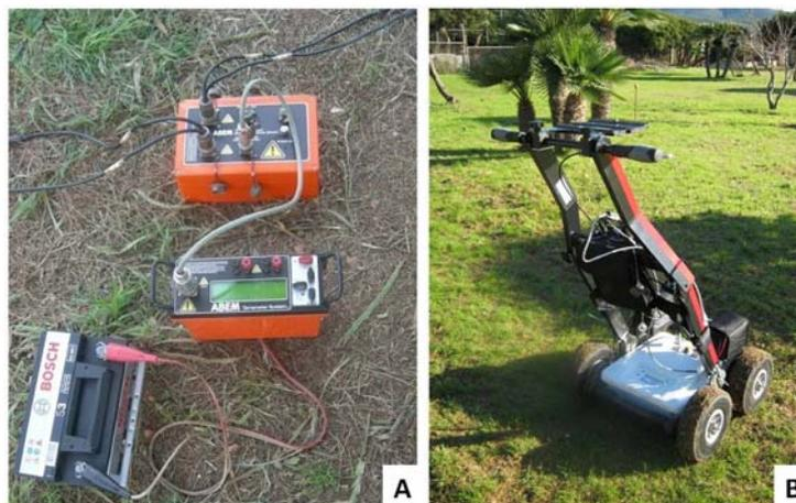
Fig. 1 - A) Abem Terrameter SAS1000 device and Lund System for electrical data acquisition. B) Ground Penetrating Radar (GPR) IDS model “RIS\_MF\_HiMod”.
