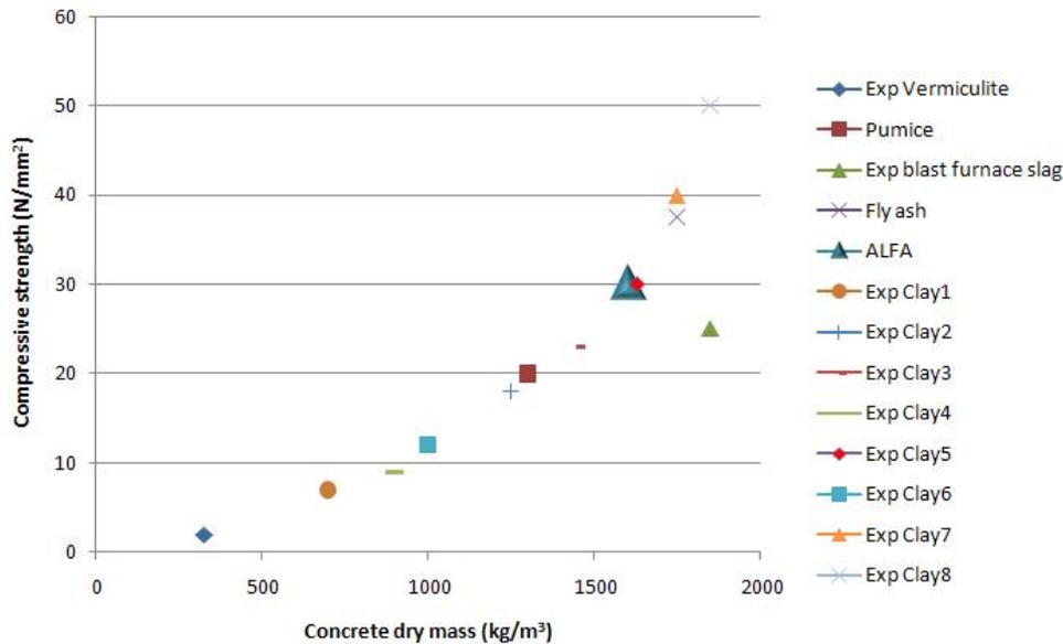
Fig. 2 - Comparison between some lightweight concretes and ALFA concrete (1Mpa = 1 N/mm<sup>2</sup>).
