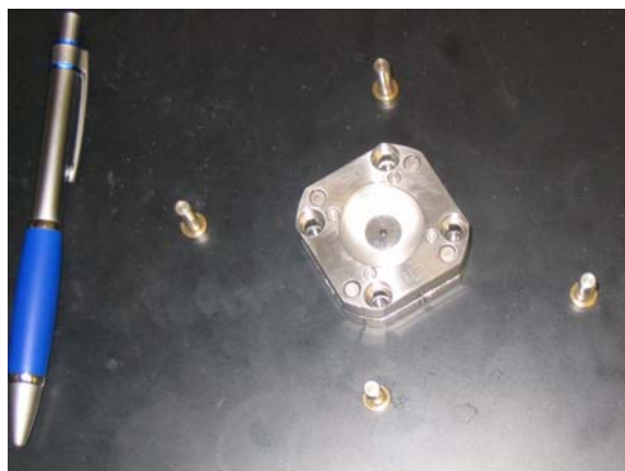
Fig. 1 - Picture of the ETH-DAC (diamond anvil cell) designed by R. Miletich (photo taken by author).
