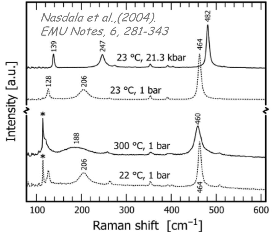
If the deformation of the structure shows elastic behavior the shift will vary linearly with the stress amplitude. Thus the Raman band position can be used to quantify stress.
