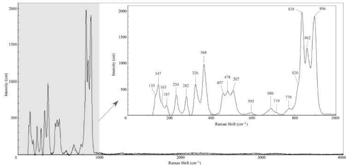
FIG. 3. Raman spectra of canosioite showing the 100–4000  $\text{cm}^{-1}$  range and the region between 100 and 1200  $\text{cm}^{-1}$  enlarged.
