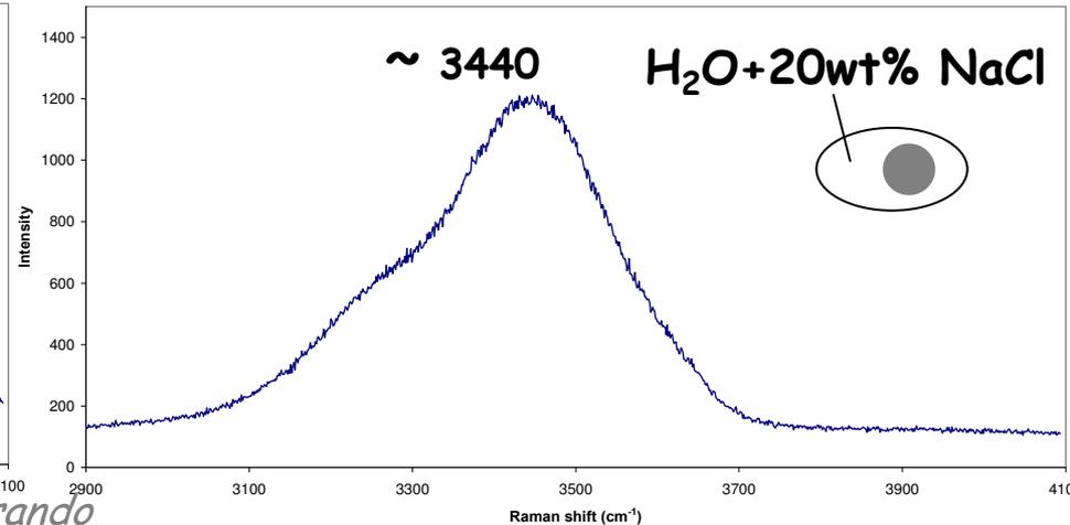
Semiquantitative estimation of the salt content, complementary to data from microthermometry, requires a specific calibration for each spectrometer
