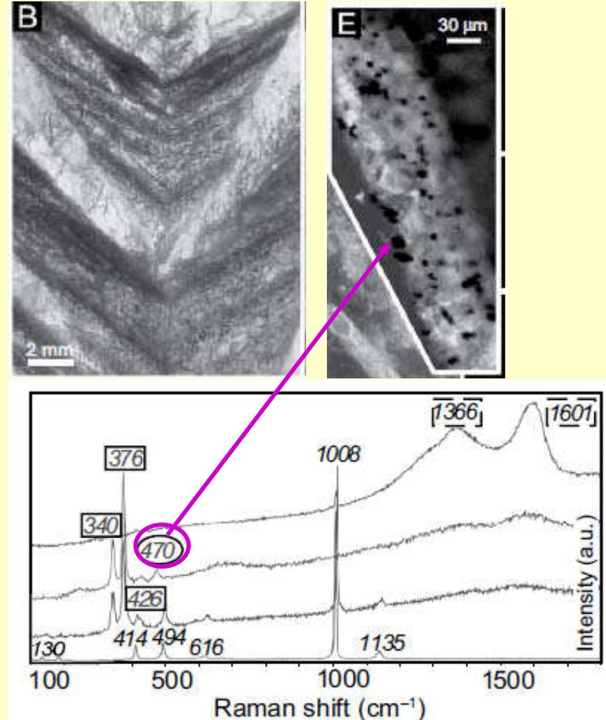
Figure 3. From the bottom to the top, Raman spectra of gypsum with filaments, pyrite (rectangles), pyrite with polysulfide (circle), and carbonaceous material (dotted rectangles).
