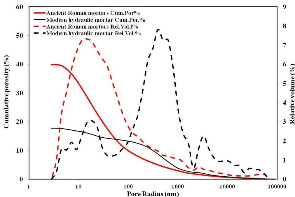
Fig. 4 - Cumulative and relative pore size distribution in Roman mortars compared with SHM (Standard Hydraulic Mortar).
